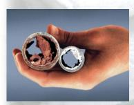
Calcium Scale is a hard thick coating or covering of calcium carbonate (CaCO<sub>3</sub>) that forms on heating elements and on the pipes and hardware of plumbing systems. As the calcium rich water enters
